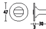
771/2531 Bathroom turn on concealed fixing rose for use with knob handles. Finishes: SS • PS • GT • BT • MA
